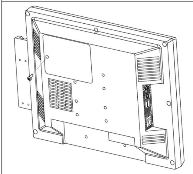
e. Loosen the screw on the cover of the hard disk bay to remove the cover.
