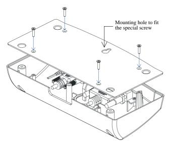
6. You may use the enclosed mounting screws (one Special screw and two Wood screws) to fix the Display on the wooden table surface.
