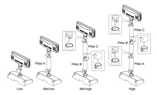
3. Insert the tab on the Display (or the extension Pillar) into the hole on the Stand until you feel it clicked.
