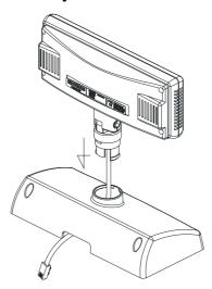
4. Connect the cable from the Display to the RJ connector (TO DSP) inside the Stand until you feel it clicked. Also connect the enclosed D-connector cable (CABLE TO PC) to the "To Host" connector and plug the power cable (POWER CABLE FROM PC) into the DC Jack (DC 12V) and connect the optional Printer D-connector cable (CABLE TO PRINTER) to the "To Printer" connector when needed.
