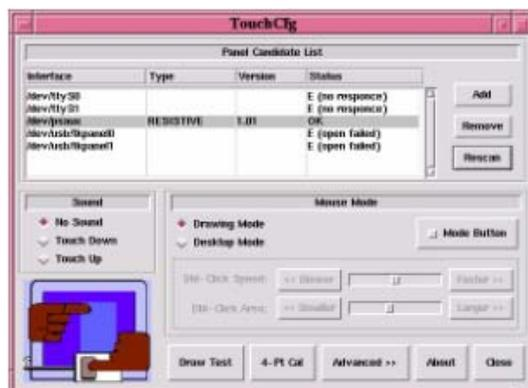
The **Panel Candidate List**, which contains by default two RS232, one PS/2 and two USB devices, commands **TouchKit** driver which port to probe for controller. If a port is occupied by other device, e.g. **/dev/ttyS1(COM2)** is used by a mouse, it is recommended to **Remove /dev/ttyS1** from the list, since the probe process would interfere the operation of mouse.
